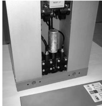
4. Dryer with front fascia panel removed.
